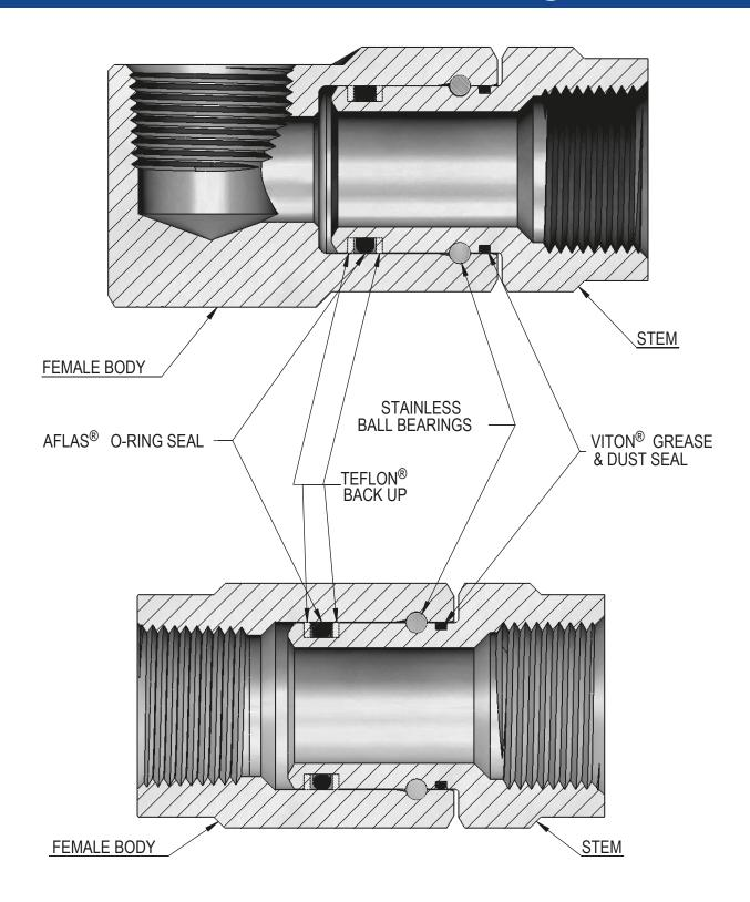
Nickel Plated for Corrosive Media Applications Sizes 4 through 16
